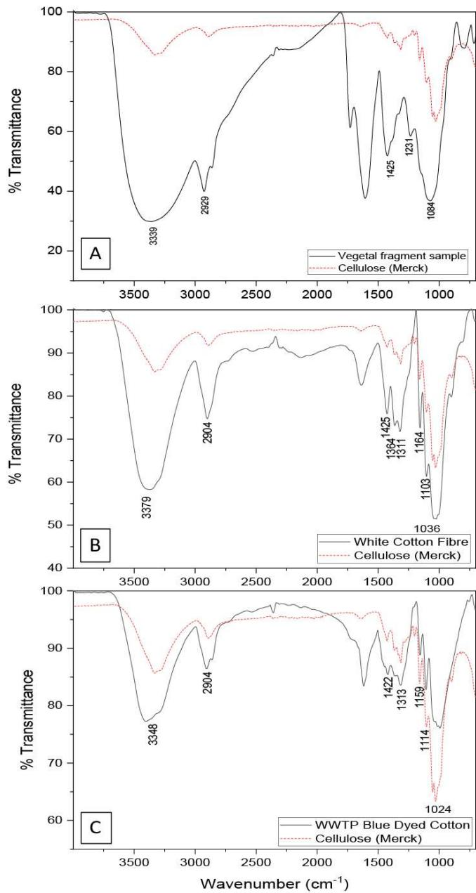
Figure S3. Infrared spectra of cellulose-based particles. A. Vegetal fragment. B. White cotton fibre. C. Blue-dyed cotton fibre.
