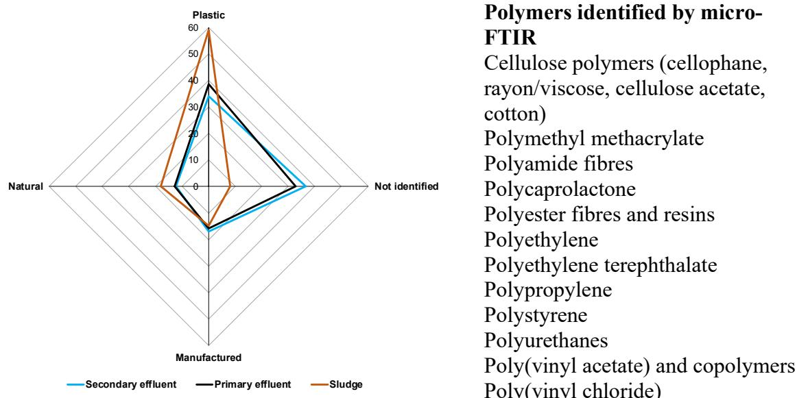
Figure S1. Distribution of materials present in the different samples after FTIR analyses. “Manufactured” refers to natural substances with evidence of anthropogenic modification and list of main polymers identified by micro-FTIR.
