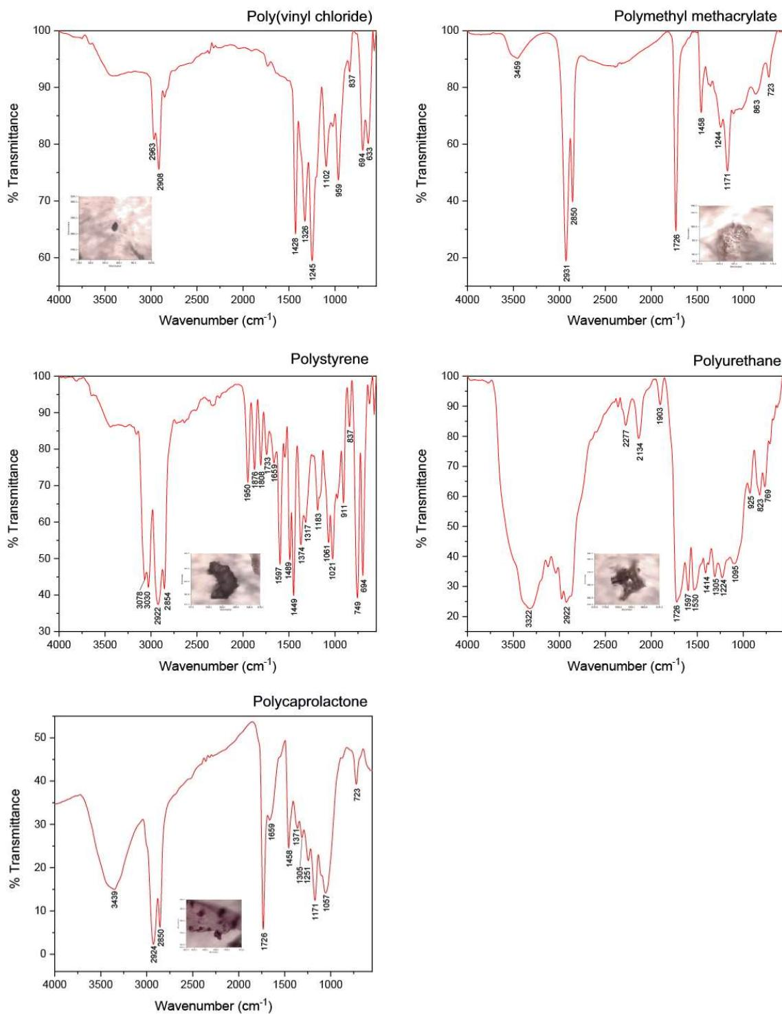
Figure S2. Infrared spectra of samples of poly(vinyl chloride), polymethyl methacrylate, polystyrene, polyurethane and polycaprolactone.
