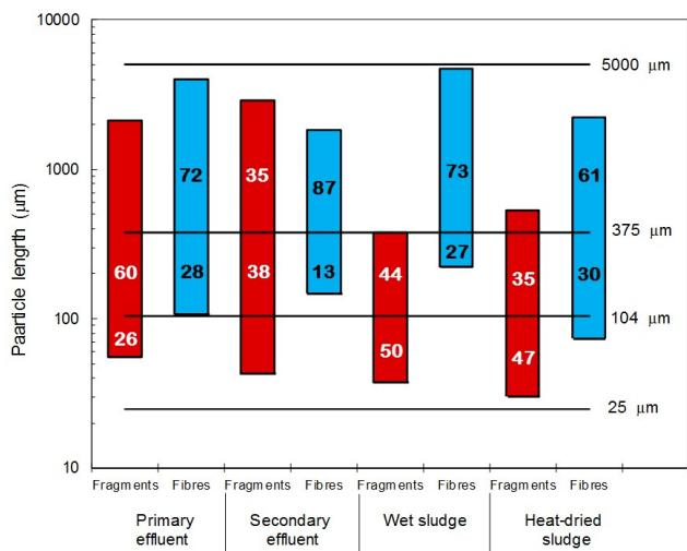
**Figure 2.** Range of sizes (length,  $\mu\text{m}$ ) in primary and secondary effluents and in wet and heat-dried sludge. (The numbers represent percentages of abundance within each category.)
